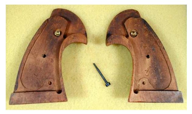
2nd gen Python grips, back. Note the fitting pads along the rear edges and the pin holes.
