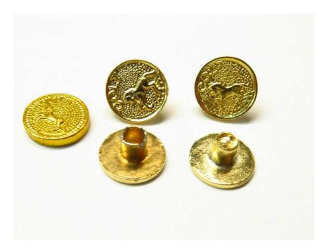
Some reproduction medallions of different origin. The one to the far left is a simple, glue-in type with an odd, concentric pebble pattern. The other ones look fairly good at first glance, but you can still tell that they are cheap castings. The one in the bottom right corner is so poorly cast that the stem is not even hollow. This means that it can't be staked, and many times you will find these glued in.
