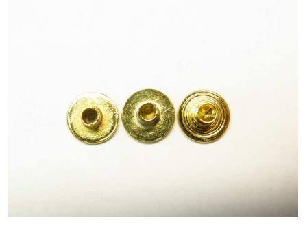
Two reproductions to the left and an original to the right. The difference in diameter is not very noticeable in the picture, but will become obvious once you try to install them. The one to the left is too small and will leave a gap around the perimeter, the one in the center is too large and won't even fit in the recess.
